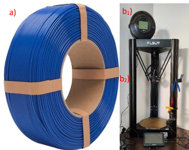
Figure 2. a) PLA+ – Blue material; b1) SUNLU FilaDryer S2 b2) FLSun v400
